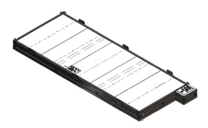
The Belly Tank is a special integrated fuel tank designed to be positioned at the base of the generator set, serving both as a structural support and a fuel reserve.
